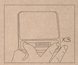
When power on in full digits 8888 press and hold the TIMER button, at the same time press the ON/OFF button for 3 times quickly.
